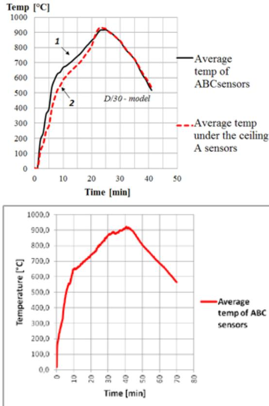
Values of monitored parameters were recorded by measuring panel type Almemo 5690-1 with K-type thermocouple. Inside the space is located 15 thermocouples. Thermocouple and compensating cable were connected to the control panel ALMEMO 5690-1. Registration of temperatures was carried out in 2-second intervals.
