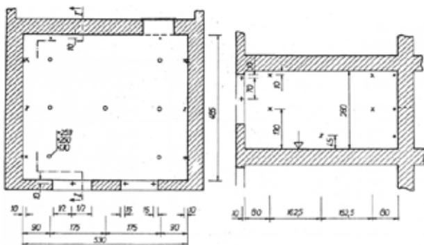
Model at scale are designed. The model with 1400mm×1300mm floor and 750 mm height (inside dimensions)<sup>12</sup>. The inner walls of the model were covered with mineral wool 5 cm thick (Figure 2). The material was found out thanks to fundamental relations of scaling. Mineral wool was
