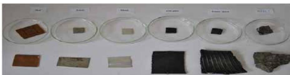
Nitric acid solution (65%) in amount of 2 ml was applied in the each sample of fuel, fluids (Fig.1). and solid materials (Fig.2). In the case of a fuel tank and fluid that was a 1: 1 and 1: 5 (5 parts by fuel and 1 part  $\text{HNO}_3$ ), and the oil was still a ratio of 13: 1 (13 parts of oil, and 1 part  $\text{HNO}_3$ ). Subsequently, the changes in temperature and pH of the solution as well as the reaction were tracked.
